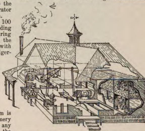
Fig. 273. Creamery with ice refrigeration.
